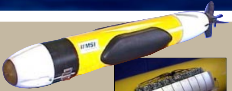
Curved ACOMMS array and sidescan sonar mounted to REMUS vehicle for Woods Hole Oceanographic Institution.
